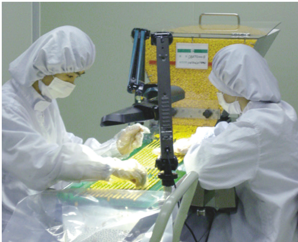
Manual sorting is labor-intensive and is limited by the speed of its operators. (Source: Proditec)
